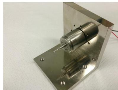
Fig. 8 120kHz type ultrasonic atomizer (SJ120kD04-1)
