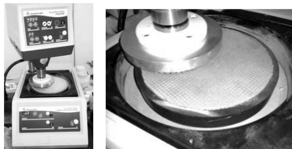
Fig.5 Lapping test machine
